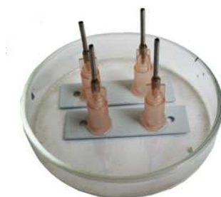
Fig. 1.2: The mechanical part of the thermodynamic flow sensor in LTCC technology (without temperature sensors)
